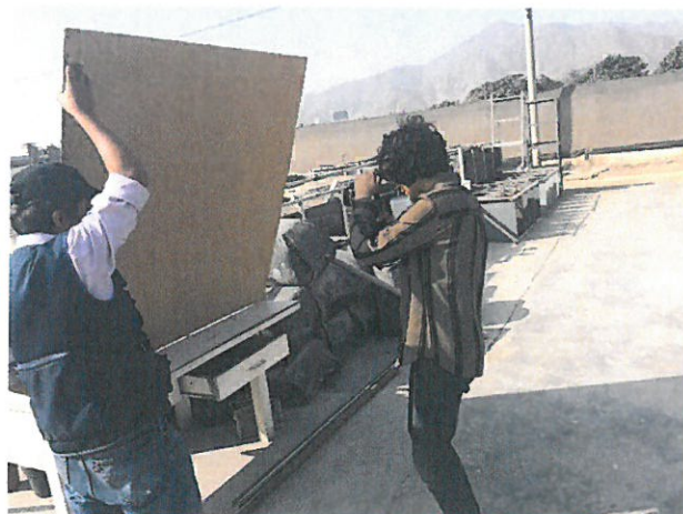
Mr. Javier Rinza (left) and myself (right) using a cardboard box as a calibration trial using infrared thermography with FLIR cameras.
