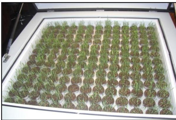
Figure 2. Rice seedlings of 13 varieties in Petri dishes on a thermogradient plate.
